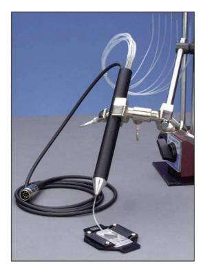
Multi-line in-line solution heating is the simplest and most effective method of warming multiple perfusion solutions to the same temperature.
