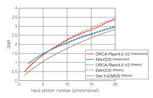
The ORCA-Flash4.0 V2 SNR exceeds that of EM-CCDs at about 6 photons/pixel. The solid lines show measured data at 533 nm. This measurement aligns well with predicted values (dotted line) for EM-CCD and ORCA-Flash4.0 V2. For comparison, the theoretical line for the Gen I type sensor is shown. Due to low QE and higher read noise, the Gen I camera does not compete with EM-CCD or Gen II ORCA-Flash4.0 V2 at these low light levels.
