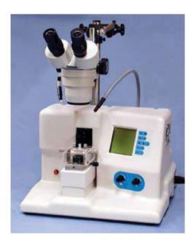
IntegraSlice is controlled using sealed Liquid Crystal Display (LCD) with associated membrane keypad to set the cutting parameters of blade speed, advance speed and section thickness. There is a rotary brightness control for the cold light source. The IntegraSliceTM operation is commenced by actuating the two-stage footswitch. The first stage starts the oscillating blade and the second stage starts the advance of the blade.
